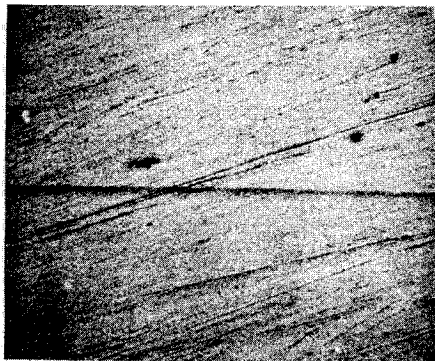
Fig. 4 Typical polished brass surface before peening with glass beads (surface character magnified \times 1000 ).
